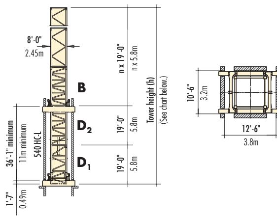
Key: **B** = Reinforced tower section - **D<sub>1</sub>** = Bottom half of D section with hydraulics - **D<sub>2</sub>** = Top half of D section
