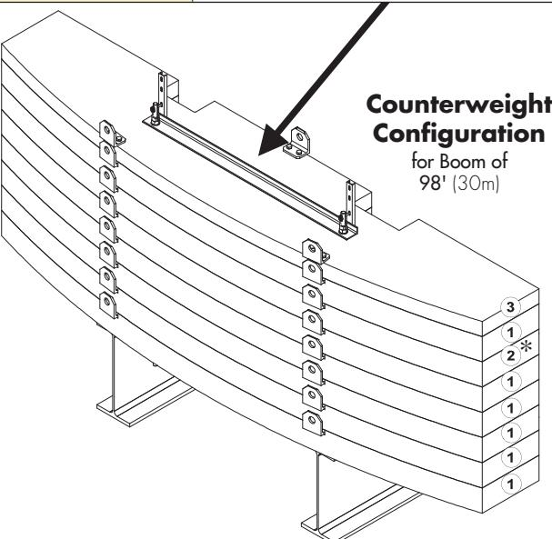
**\*IMPORTANT:** Six (6) counterweights must be installed and secured before the boom is attached. Ballast blocks **②** with fastening plates secured in the openings shown must be in the sixth position.
