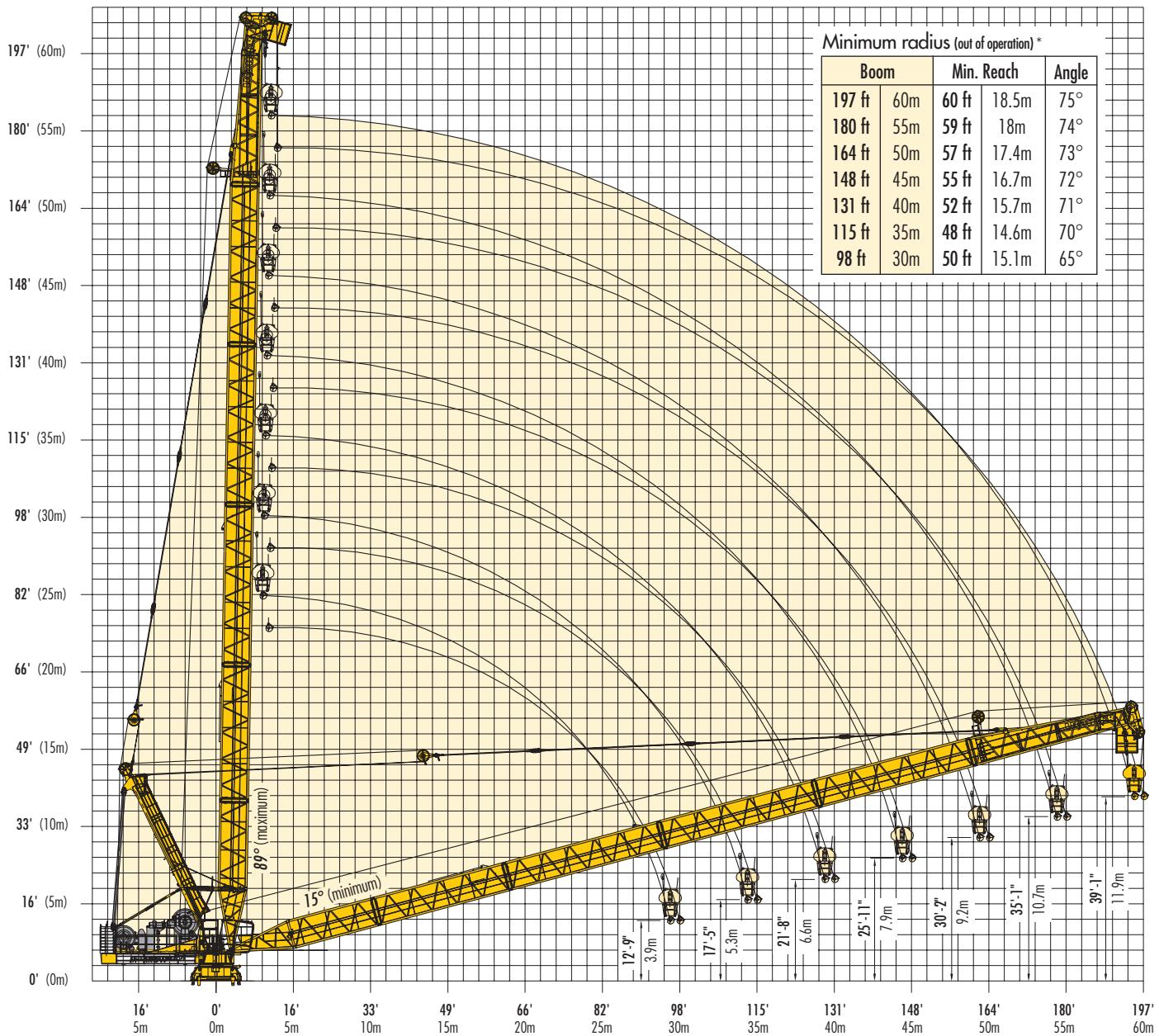
\* NOTE: Out of operation boom position from 15° to 70°. Out of operation boom position dependent on boom length and number of tower sections installed.
